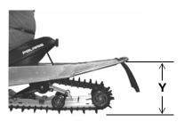
To determine sag, commonly referred to as ride-in, subtract measurement Y from X (Sag=X-Y). Adjust sag by rotating the torsion spring preload cams located on the rear torque arm. See illustration. The ideal amount of sag for this rear suspension is five inches (12.7 cm) (X-Y=5 in./12.7 cm).
